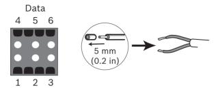
Figure 5.9 Data connector pins
